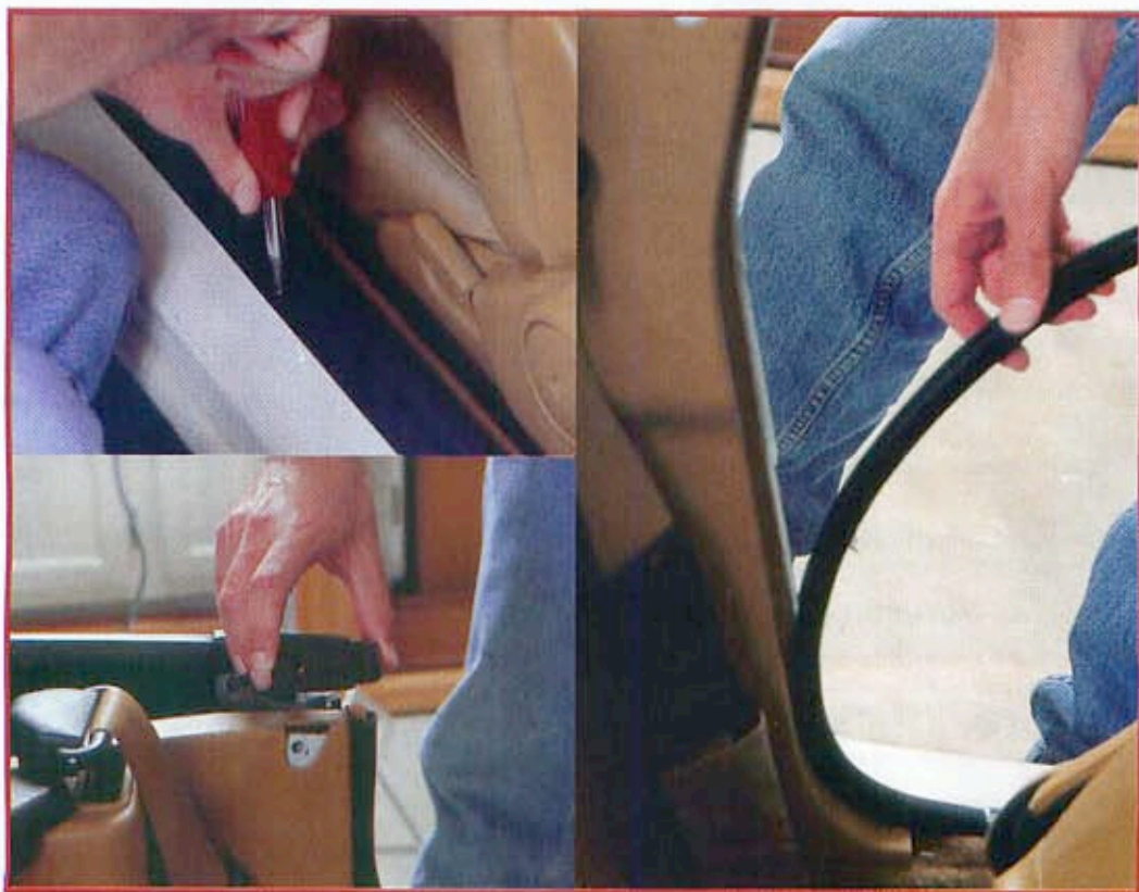
1) Begin the installation by removing the doorsill scuff plates, the beltline cover trim, and the door seam seal.
