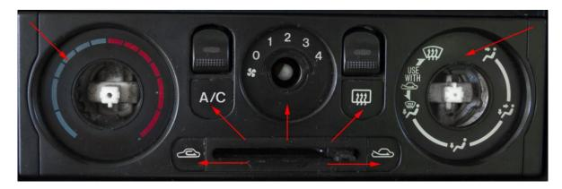
The plastic covers are glued to the heater panel. To remove them, you can use sharp utility knife/cutter and a small flat screwdriver. Gently slide the cutter along the edges until it is positioned below the plastic cover and carefully lift upwards.
