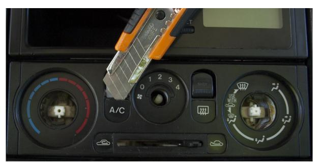
*Important*: After removing them, peal/clean the remaining glue. You can use a small flat screwdriver to peal the remains of the glue.
