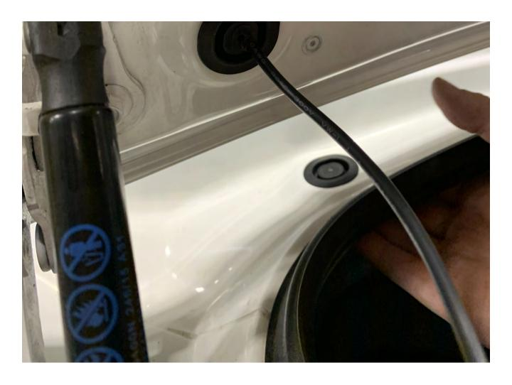
Remove the rubber plug on the body of the car just in front of the trunk weather stripping and perform the same treatment.
