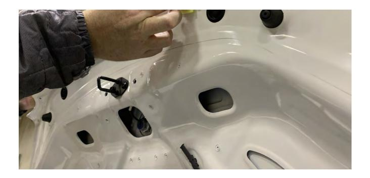
Peel the backing from the adhesive on the LED light strip and affix it along the underside of the trunk lip. Apply it in approx 6 inch increments.
