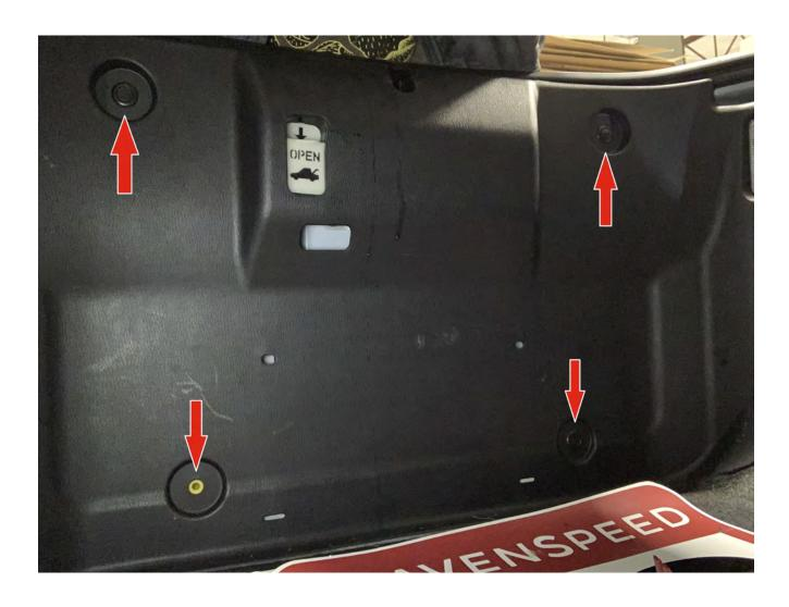
Next, pull the four drivers side trunk clips so you can peel the carpet back and see the wiring we're going to install the Y-wire connector into.
