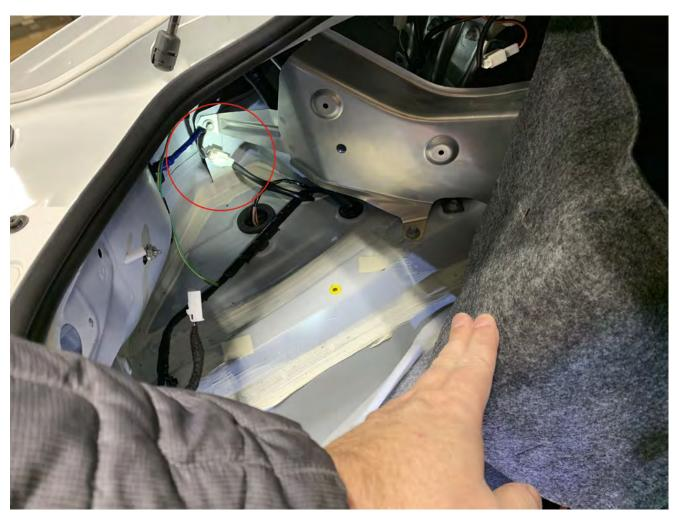
It only installs one way, so take a look at the plugs and match them up with the correct side. The two-lead plug will connect to the LED light strip.
