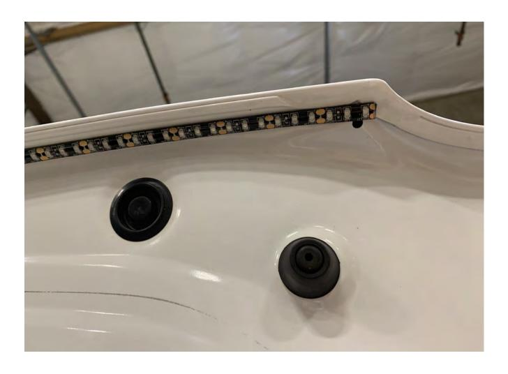
With the LED light strip completely installed, let's turn our attention to finishing up the wiring. Remove the round plastic plug that is just a few inches away from the wiring side of the LED light strip on the underside of the trunk lid.
