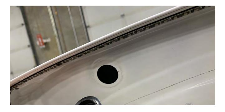
You can either drill a 3/16" diameter hole through the center of this plug or take a utility knife and cut a slit across the face of the center. If you choose to slit the cap you can then push the plug through the cap. If you drill the 3/16" hole, you will need to remove the plug from the end of the wiring.
