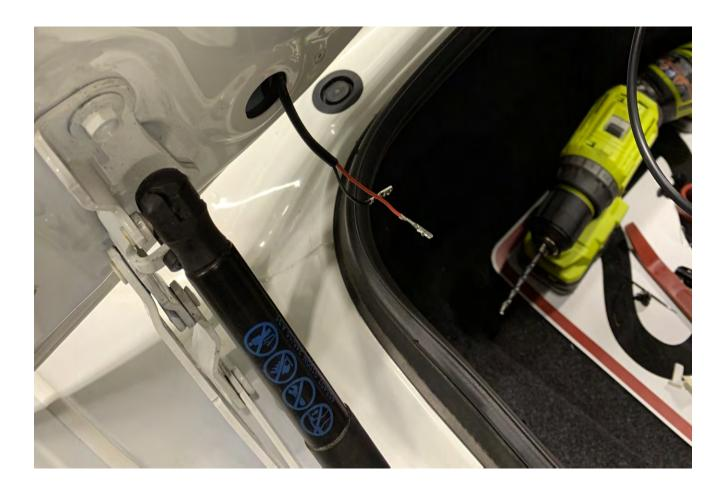
Create you wire clearance through this rubber plug and feed the wire through. Replace the plug and take out the slack in the wire through the lid interior.
