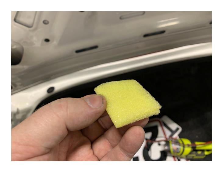
$Run\ the\ foam\ applicator\ along\ the\ underside\ trunk\ surface\ where\ the\ LED\ light\ strip\ will\ mount.$
