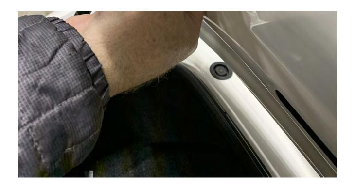
Snap the plastic plug back into place and take up the slack in the wire. Apply one of the cable tie mounts and a zip tie to keep the wire out of harms way.
