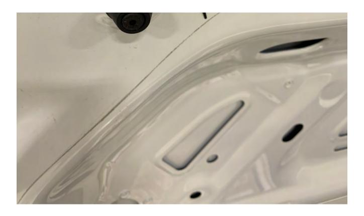
Going back to the wire now coming out of the oblong hole in the trunk lid, pull out the rubber plug in the lower left side of the lid and continue fishing the wire over and out that hole.
