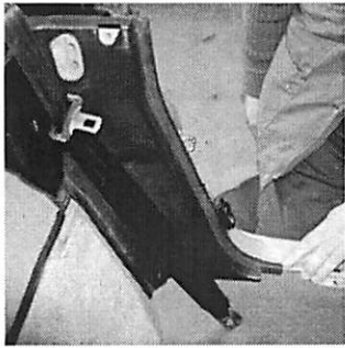
RE-FIT REAR DOOR SEALS. ENSURE THEY LINE UP AT THE TOP
