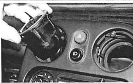
REPLACE THE AIR VENTS
