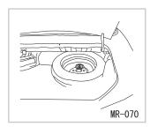
After the Rear Dampers are installed onto the car the spare tire will not sit in its original spot without putting too much pressure on the top of the Piston Rod. In order to counter this the spare tire needs to be offset as far away from the Piston Rod as possible. Using the original mounting hardware, mount the wheel using one of the lugnut holes instead of the center. This should provide ample clearance of the spare tire and Piston Rod.
