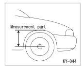
3. After installing the tires, measure the distance from the wheel center and the fender edge as shown in the Figure, and confirm that it corresponds to the reference value shown below.
