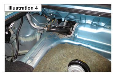
5) Using a ratchet, 3"and 6" extensions, and a 14mm socket, remove the (four) nuts securing the strut tops to the body of the car. Do not remove the center nuts that hold the strut assembly together.
