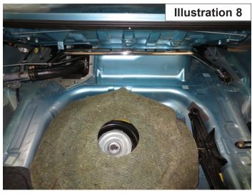
9) Try test fitting the fuel line cover panel. You'll notice the panel needs to be trimmed to be installed. Make marks on the panel using a felt tipped pen where you will trim. Remove the panel from the car and trim it using tinsnips. This may take a few test fits and trimmings to get it in place and looking good. Cut a little at a time.
