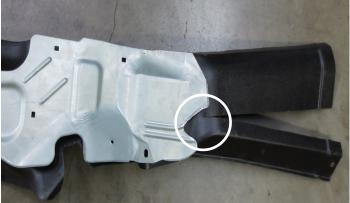
11) Reinstall the fuel line cover panel for the last time. Once again test fit the left side finish panel. This time the panel should go almost all the way on. Trim and test fit until you are satisfied with the fit and then install it for good using the push-in fasteners.
