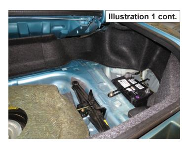
2) Using a Philips screwdriver, remove the cubby on the left side of the trunk floor.
