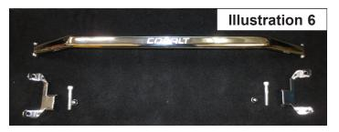
7) Set each of the strut brace end brackets over the strut top studs. The brace will only fit with the bracket offset toward the rear of the car. Start a nut onto each of the studs a few threads but do not tighten them down.
