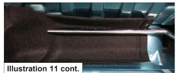
12) Test fit the right hand finish panel. Take note of the area that must be trimmed in order to fit around the
