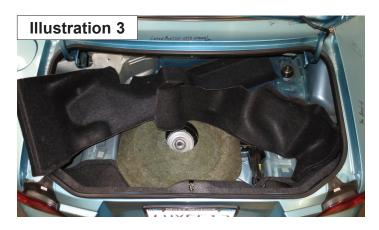
4) Using a ratchet and 10mm socket, remove the metal panel that is covering the fuel filler hoses.
