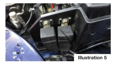
6) Unbolt both the 10mm bolt and 10mm nut connecting the plastic bracket to the body of the vehicle, then remove the 12mm nut holding the bracket to the air box.
