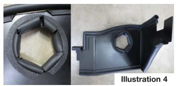
5) Position the heat shield in the engine bay. It should stay to the outside of the power steering reservoir and block off the entire corner of the engine bay behind the driver side headlight.
