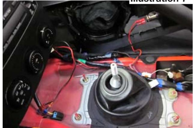
8) Before the center console can be installed for good, you must first install the lower dash and lower dash side covers. Do not forget the electrical connections. Reassemble your interior. You will end up with 4 extra screws. 3 left over that secured the old cubby to the center console and 1 that secured the center console to the car through the old cup holder. Enjoy your new Center Console Insert!
