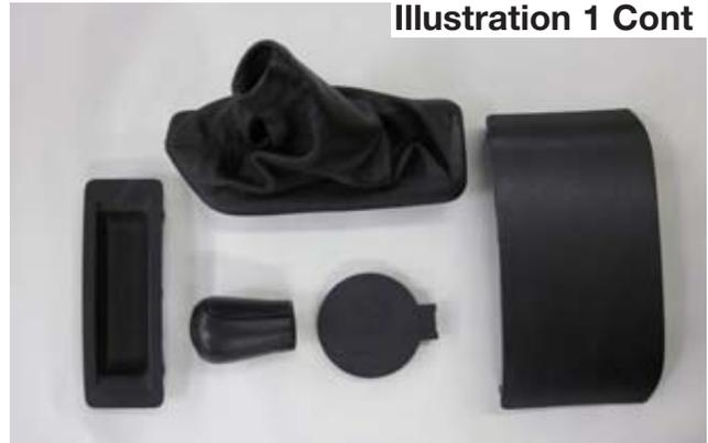
2) Use a Phillips screw driver to remove the 5 screws under the panels you removed in step 1. Slide the cup holder cover forward. Pull straight up on the front of the center console to release it from the lower dash. From the passenger side, lift the center console enough to unplug the power window switch. Remove the center console from the car.
