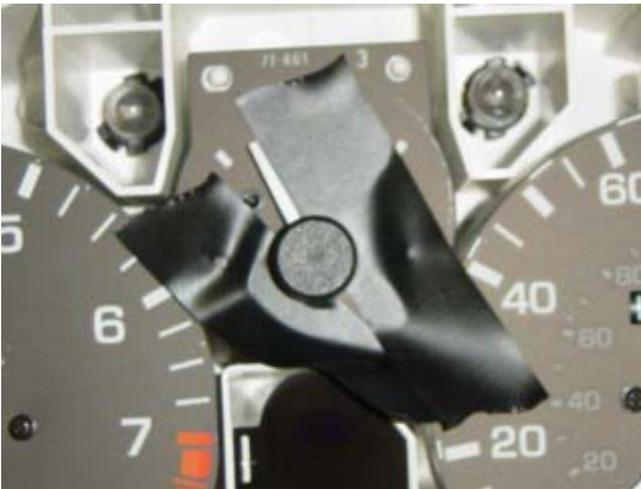
Photo 4-A: Use electrical tape on the face of the gauge panel to protect it
