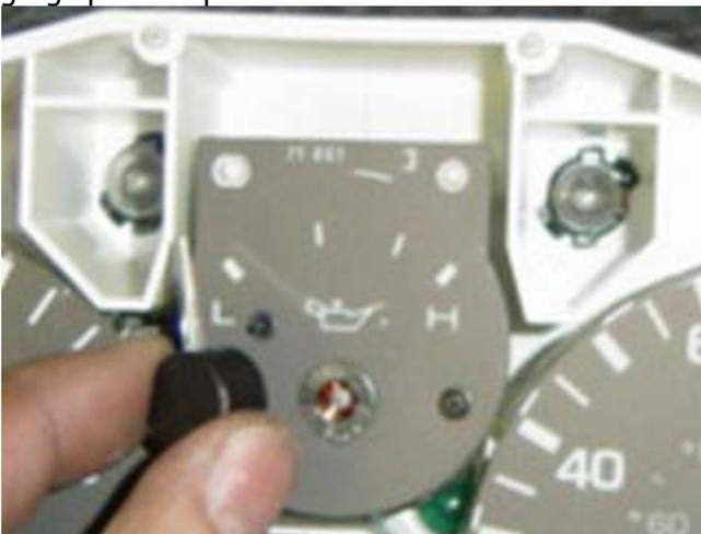
Photo 4-C: Pointer removed from the gauge
