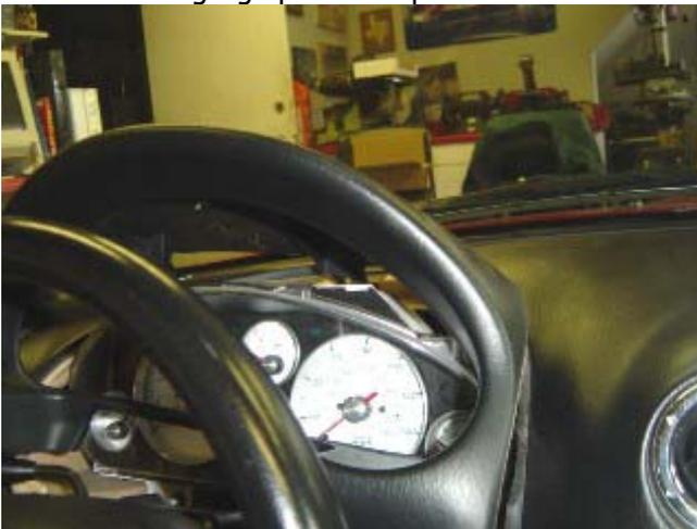
Photo 3-E: Remove bezel and set aside
