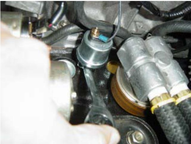
Photo 1-C: Use a 1/2" open-end wrench to tighten the new oil pressure sender
