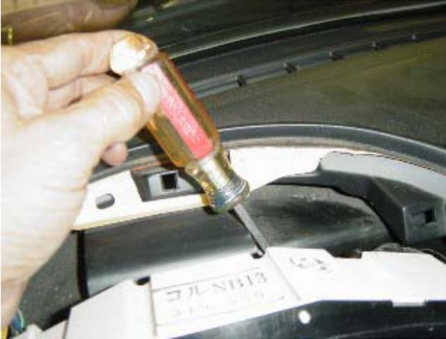
Photo 2-H: Remove the speedometer cable by using a screwdriver to press the release clip
