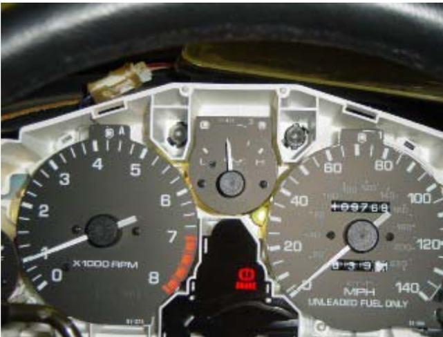
Photo 4-D: Oil pressure pointer at idle
