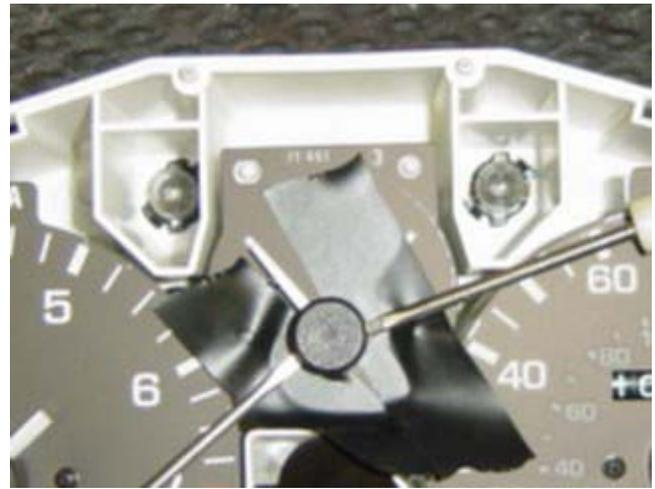
Photo 4-B: Using two small screwdrivers, apply even pressure to release the pointer
