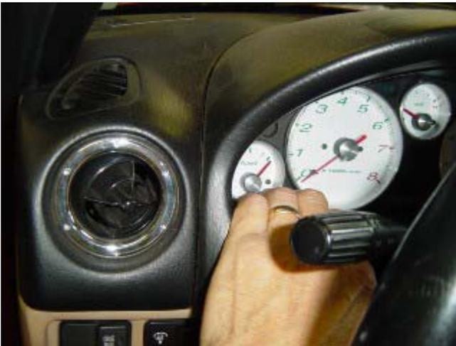
Photo 3-C: Using your fingers, reach between the bezel and the gauge panel and pull to release
