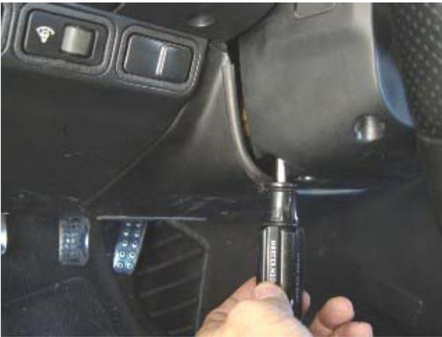
Photo 2-A: Remove the screws holding the steering column cover on with a Phillips screwdriver
