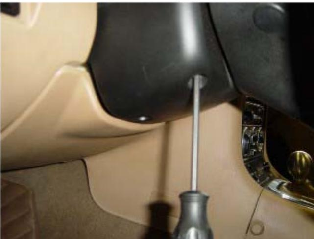
Photo 3-A: Remove the steering column cover
