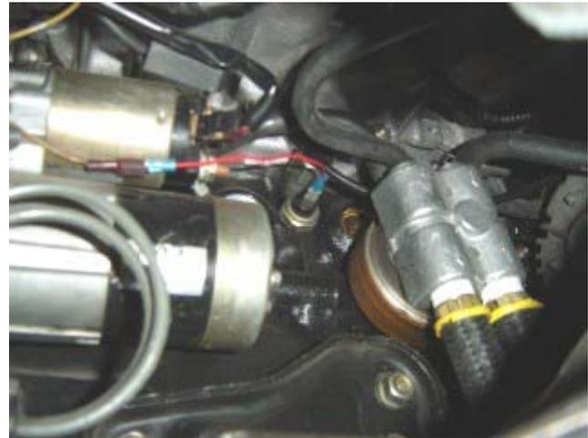
Photo 1-B: Location of the stock oil pressure sender
