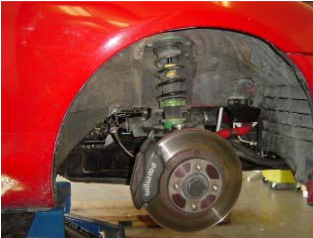
Photo 1-A: Remove the tire for access through the fender well
