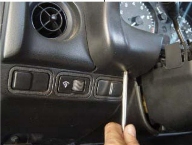
Photo 2-C: Remove Phillips screw in the dashboard bezel
