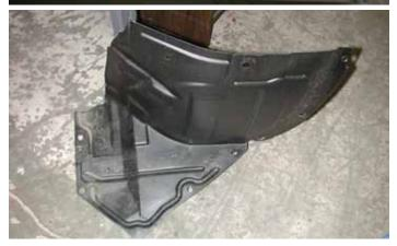
5. The larger part of the inner fender will not be removed from the vehicle. Instead, pull it down away from the body of the vehicle and let it hang. Using a 10mm socket, remove the two M6 nuts and M6 bolt on each side of the vehicle that secure the bumper cover to the body. They are located under the plastic inner fender. Disconnect the side marker and fog lights.
