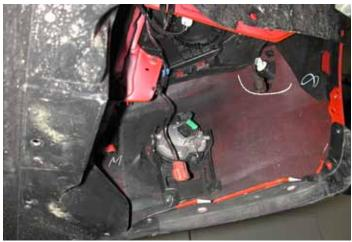
Lay a carpet or blanket down to keep your bumper cover from getting scratched. Remove the bumper cover from the vehicle by pulling it straight forward.
