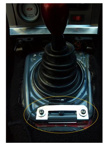
The bracket has to be adjusted this way, that the short console can slip in, while the front is perfectly aligned with the centre stack. Easiest way to achieve the correct distance is to mount the bracket loose on the fixing bolts, push the
