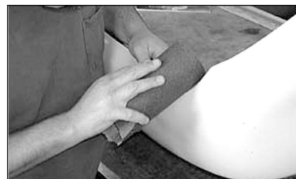
Photo 4. Finish the shape of the opening using a round sanding block.
