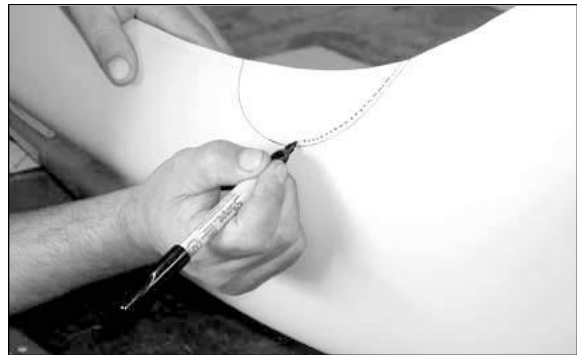
Photo 2. Mark a “dotted” cutting guide 1/8” inside the template line.
