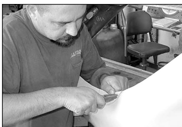
Photo 3. Making a single cut with a utility knife.
