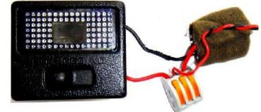
The black one of the Sun Visor Light should be now connected to the slider of the courtesy lights, using the attached ring cable lug shoe - the screw on the slider need to be used for this purpose (shown with the screwdriver on the following photo).
