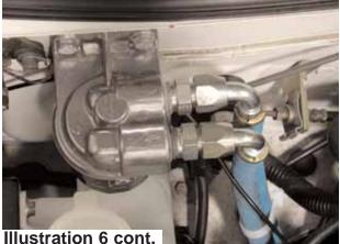
Then connect the remaining line's large straight fitting to the left top nipple on the cooler making a large gentle curve. This line will also pass under the bottom right corner of the radiator, following the right side frame rail backward to the IN nipple (center most) on the Engine adapter plate, finger tighten only.
