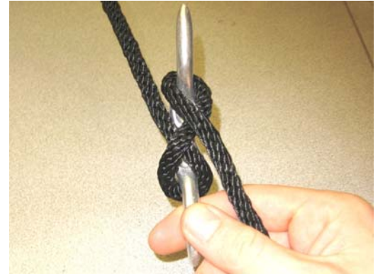
Fig. 10 – Tie Cleat, Step 1
