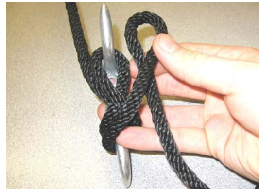
Fig. 11 – Tie Cleat, Step 2
