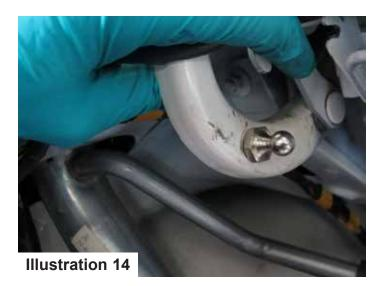
15) Move the hook up and out of the way and attach the free end of the strut to the ball stud.
