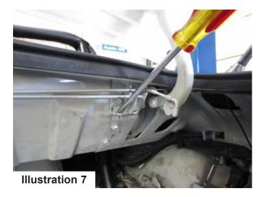
B) Using the two supplied bolts and star washers, attach the trunk lift bracket and spacer in place of bolts removed in step 3. Ensure the narrow section of the
