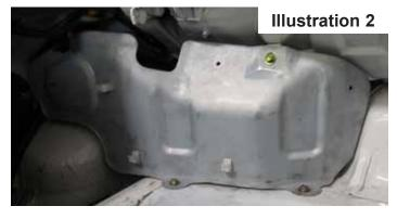
Remove the two bolts found directly behind the left trunk hinge. These bolts will not be used in the installation of the trunk lift.
